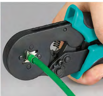
Put the stripped insulated conductor into the terminal
