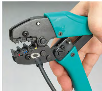
Press gradually and crimping well
