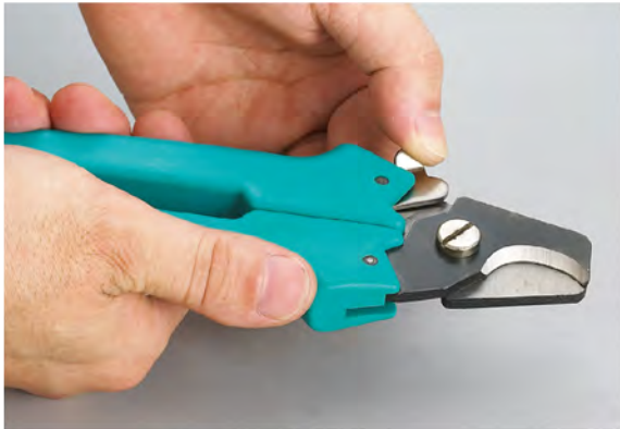
Open the hand paddles to start cutting.
