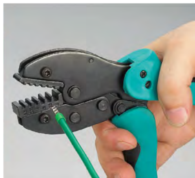
Press gradually and crimping well
