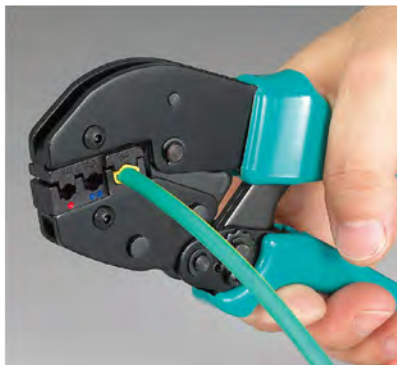
Put the stripped insulated conductor into the terminal
