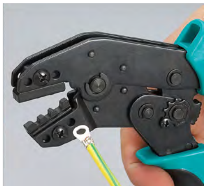
Press gradually and crimping well
