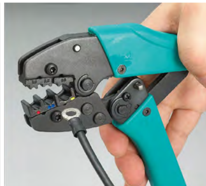
Press gradually and crimping well
