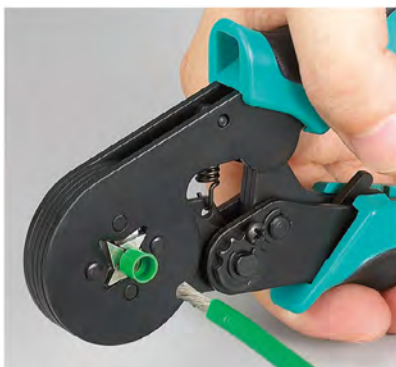
Put the terminal in die set firstly
