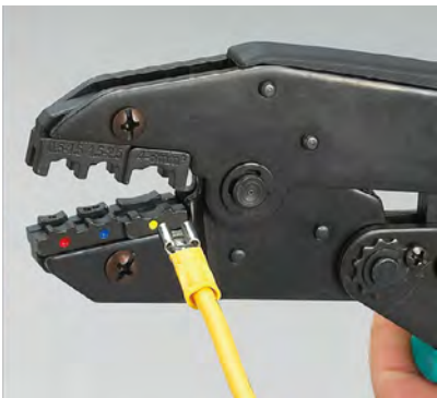
Press gradually and crimping well
